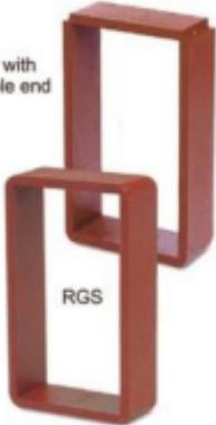
RGS is standard frame for marine application; it has a standard internal width of 120 mm, 10 thickness and 60 mm deep. There are four sizes of RGS, denoted by 2, 4, 6 and 8 depending on their height. They may be used in both vertical and horizontal multiple frames.
